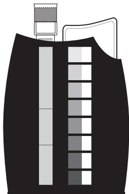
The Octa-Slide 2 Viewer should be held so non-direct light enters through the back of the Viewer. Insert the Octa-Slide 2 Bar into the Viewer. Insert the reacted sample into the top of the Viewer. Match the color of the reaction to the color standards.
